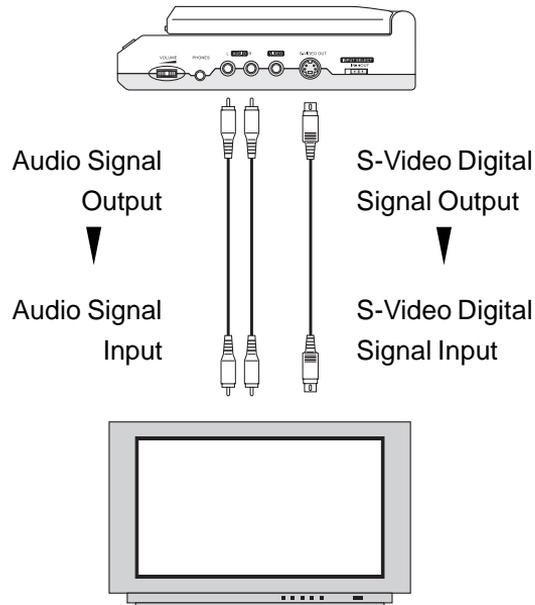
Certain AV equipment (e.g., high-end televisions and VCRs) include an S-Video input port. In this situation, you may use the included, or purchased, 4-pin S-Video signal cable in place of the yellow video cable. Using the S-Video cable should provide superior picture quality.
